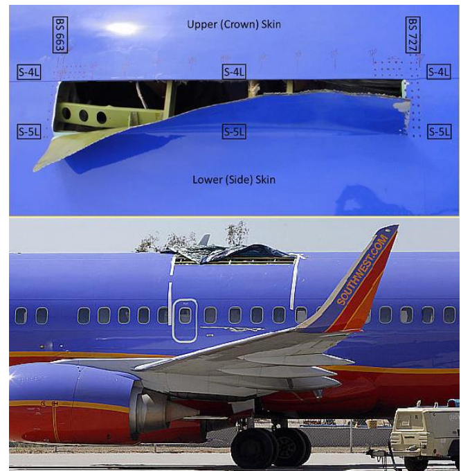
Fig. 42. Roof of the Boeing 737-300 Southwest Airlines Flight 812 with 1.5-m long rip, April 1, 2011. Source: https://www.scientificamerican.com/article.cfm?id=southwest-airplane-aluminum-cracks .
