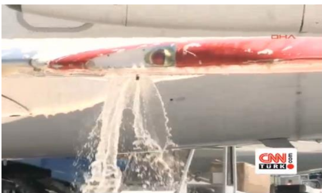
Fig. 45. Fuel leakage from the damage tip wing of the Tu-154M RA-85799 at Istanbul Ataturk airport on July 27, 2011. Source: http://www.euromag.ru/turkey/11679.html
