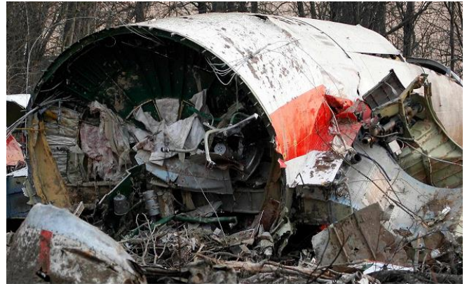
Fig. 26. Rear part of fuselage of the Tu-154M PLF 101 torn around the frame No. 65 with broken bolts.
