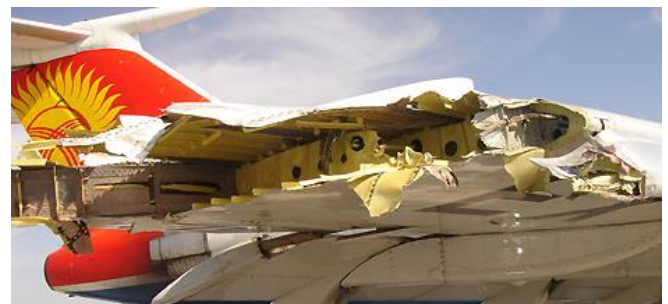
Fig. 11. Details of the damaged right wing of the Tu-154M EX-85718, which struck the parking KC-135R tanker.
