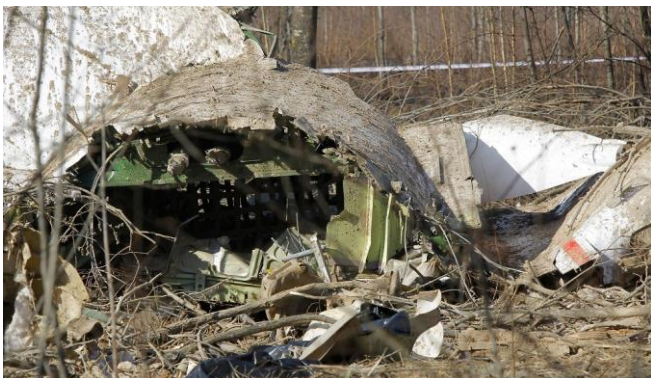
Fig. 25. Split skin of the fuselage (resting upside down) of the Tu-154M PLF 101 along its longitudinal axis and rolled out.
