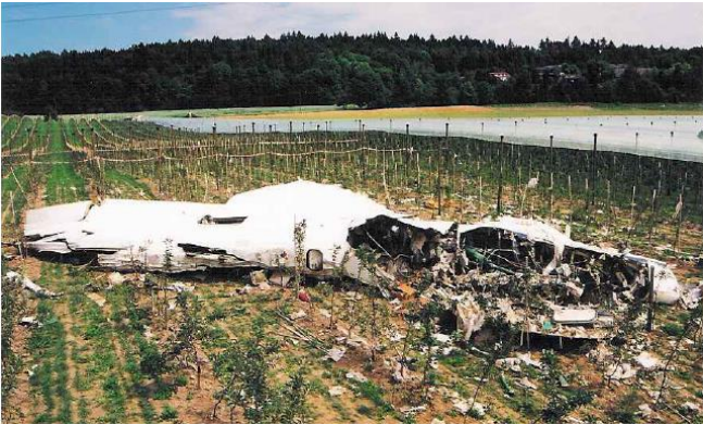
Fig. 5. The forward fuselage section of the Tu154M RA-85816 (Uberlingen mid air collision July 1, 2002) found at apple plantation near Brachenreuthe (Lake Constance) [6].
