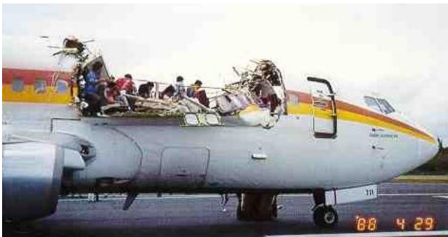
Fig. 41. Open fuselage of the Boeing 737 Aloha Airlines, Flight 243, April 28, 1988 due to cracks along riveted paths. Source: http://deicinginnovations.com/wp-content/uploads/2012/07/Aloha.jpg
