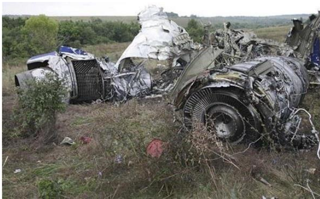
Fig. 24. Turbofan engines Kuznetsov NK-8-2 of the Tu-154B2 RA-85556 on the crash site.
