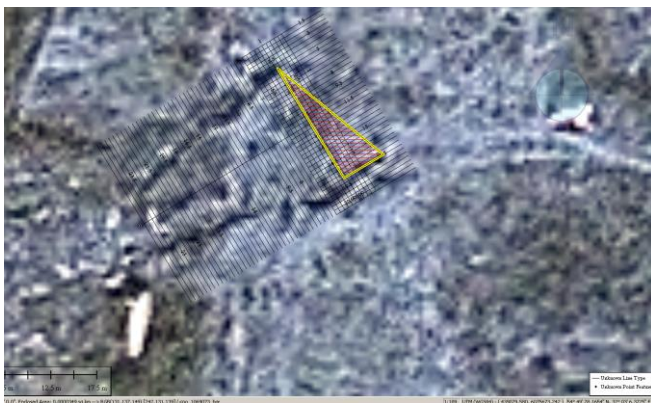
Fig. 9. Satellite photo of ground traces from 11-th of April 2010. The upper groove is the trace formed by the left wing and the lower trace the groove formed by the tail contact. The length X_{wt} = 15\text{ m} , of the hypotenuse of the drawn triangle is equal to the distance between the initial wing contact and initial tail contact. The short triangle leg is parallel to the plane movement prior to ground contact. The length defined as X_p = 5\text{m} .
